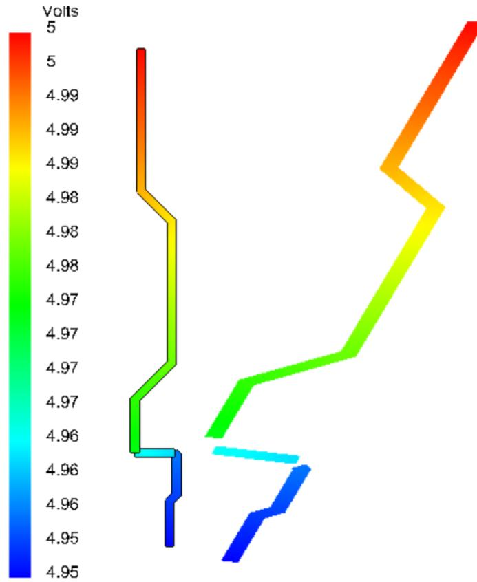
The separation in the traces shown above-right, is where the electrical vias. Below shows the elements. The vertical lines are the Resistor elements representing the vias.
