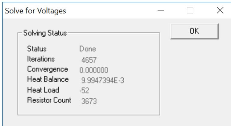
After solving for voltages, the Boundary Nodes and the Nodal Heat Loads are deleted from the model. All trace Properties are automatically changed to reference the material defined for the metal layers.
