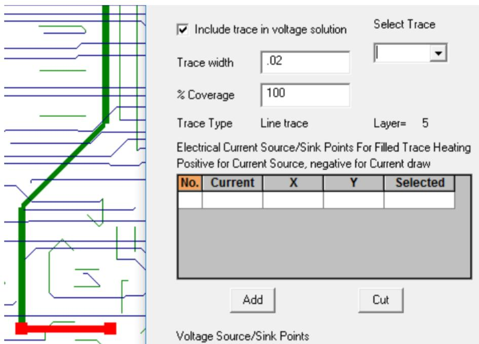
The screenshot shows a PCB layout on the left with a green trace on layer 5 and a red trace on layer 1. A dialog box on the right is used to configure the selected trace. The dialog includes the following fields and options:
