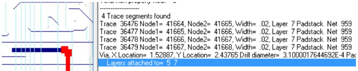
So in this case, the current applied to the trace on layer 7 will travel through the via to the trace on layer 5. It will travel down the trace on layer 5 and through the via connecting the trace on layer 1 to the voltage at the other end of the trace on layer 1, completing the circuit.
