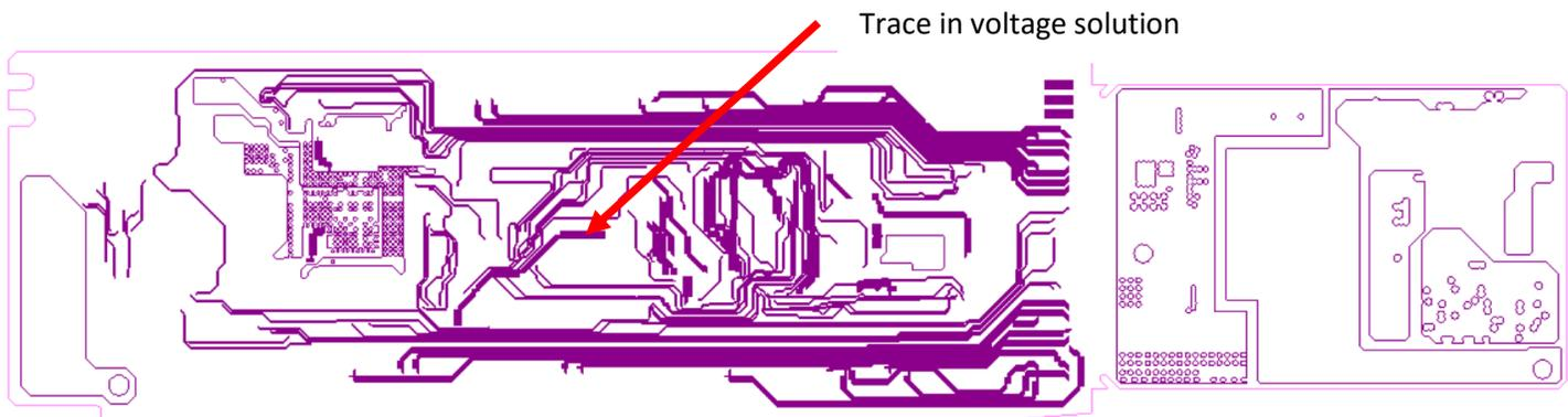
The four traces shown above will be explicitly meshed in the board. Below are shown Solaria Line elements that were generated from the traces selected.
