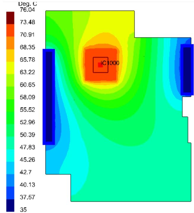
To see the effect of only the Joule heating in the traces, in the property for the component, the power was changed to zero and the model was re-solved.
