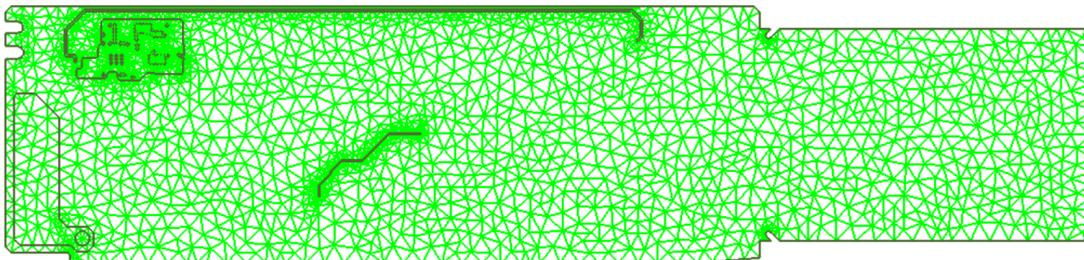
When the board is meshed, each trace references its own Property. The elements generated are on the same layer in the model the actual trace is on.
