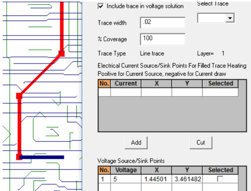
To make sure that the traces on the different layers will be electrically connected, select Information>Element. Make sure Vias are viewed in PCB>View Entities. Hit Select then click on the intersection of the two traces, as shown below. In this case it shows that the via is connecting layers 1 and 5. Therefore these two traces will be electrically connected in the voltage solution.
