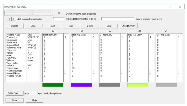
Shown below is the array that is referenced. You can see that the heat transfer coefficient is a function of the temperature difference between the board surface and the air. During the solution, this data is used to calculate the appropriate heat transfer coefficient based on the board and air temperatures.
